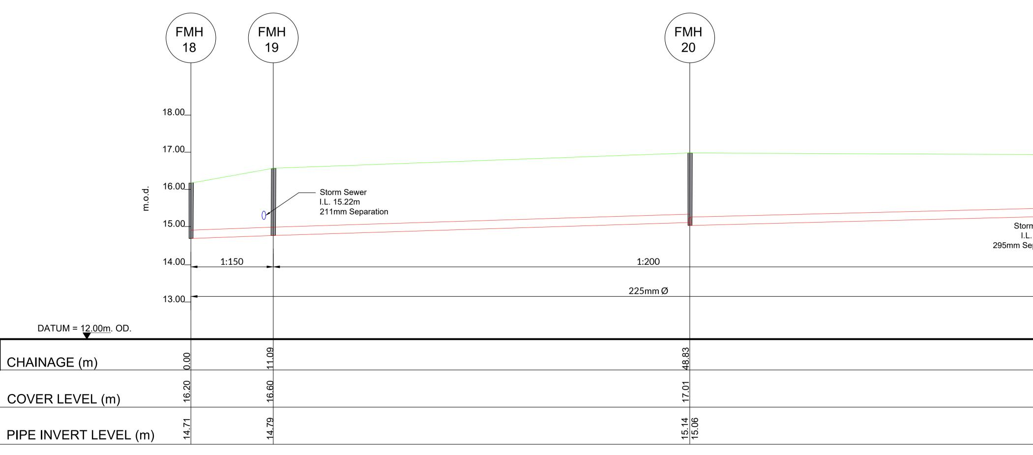
Foul Sewer Longitudinal Section FMH 18 - FMH 21 Horizontal Scale = 1:250, Vertical Scale 1:50
